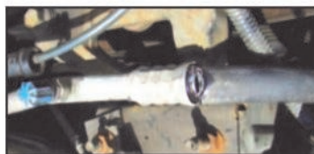
PROBLEM — Damaged A/C hose leaking at connection
