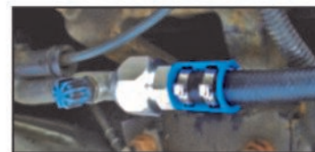
PROBLEM SOLVED — With hose to compression union adapter
