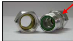
PROBLEM - Damaged A/C hose leaking at connection
