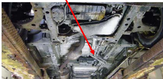
PROBLEM - Damaged Rear A/C line or component
