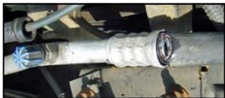
PROBLEM - Damaged A/C hose leaking at connection
