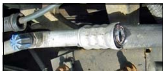
PROBLEM - Damaged A/C hose leaking at connection
