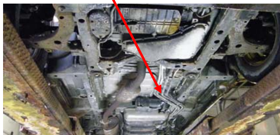
PROBLEM - Damaged Rear A/C line or component
