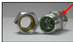
PROBLEM - Damaged A/C hose leaking at connection
