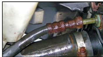
PROBLEM - Leaking transmission line connector
