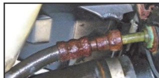
PROBLEM — Leaking transmission line connector
